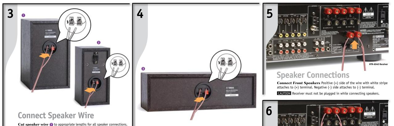
Connect speaker wire for front speakers (1), and surround speakers (2). The positive (+) side of the wire with the white stripe attaches to the red terminal. The negative (-) side attaches to the black terminal. (See your HTR-6040 Owner's Manual for more information on speaker wire connections.)
